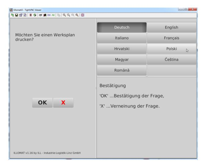
The driver can now confirm or deny entry. In the next step, the loading papers are printed. Boom gate 2 remains closed.
