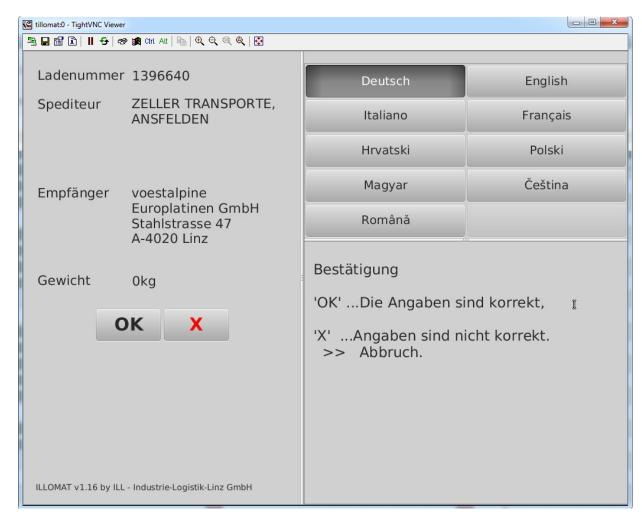
The weight is checked. It is verified whether the weight exceeds 40 tons (tare weight + weight of the load). If the weight is over 40 tons, an overload confirmation must be present, which must be uploaded in advance by the freight forwarder (PDF). The program does not check the content of the PDF! This will be manually checked later in the hall.
