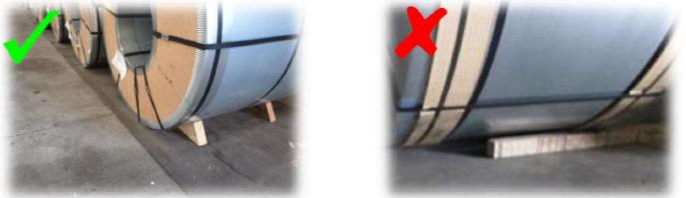
Figure 2: Securing of coils during interim storage
