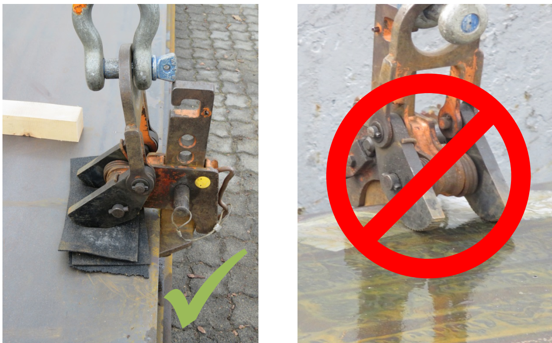
Figure 2: Suitable use of safety clamps for handling of heavy plates
